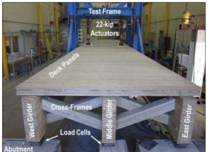
Figure 3. Glulam girder bridge test specimen. (Photo credit: Mostafa Tazarv)
