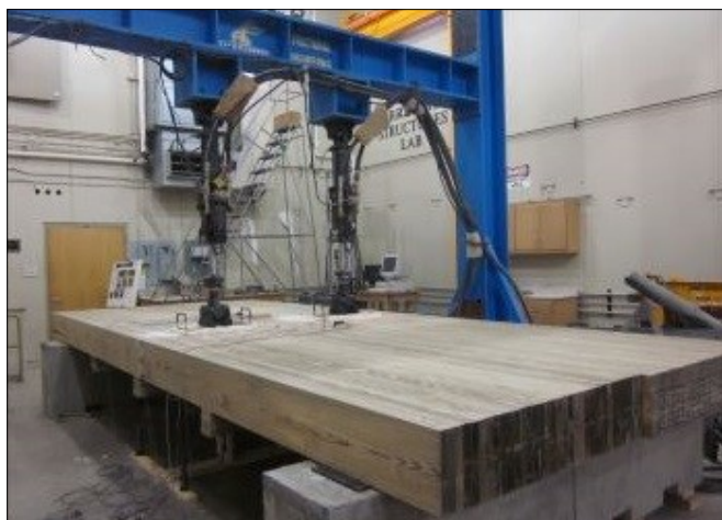
Figure 4. Glulam slab bridge test specimen. (Photo credit: Zach Carnahan)
