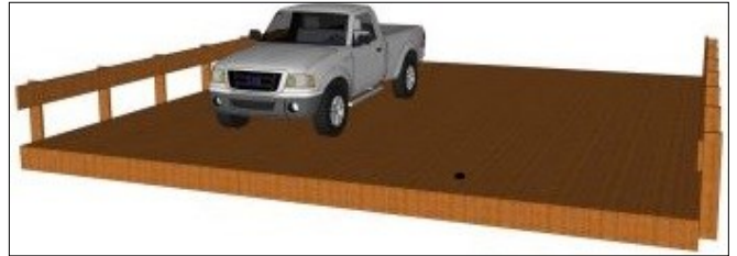
Figure 2. Glulam slab timber bridge. (by: Zach Carnahan)
